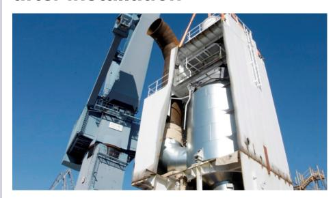
SCRUBBER PIPEWORK IS having to be replaced less than six months after installation because of corrosion problems that experts have told Lloyd's List is almost impossible to predict, and not widely understood by either shipowners or installation teams.
